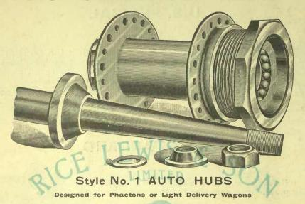
The Wire Auto Wheel has come to stay, owing to the many advantages offered. Our Auto Hub are designed and have proven to be as easy running as any bicycle hub. The cups, cones, axles an shells are all turned from the best material obtainable. These hubs will carry a gross weight of  $5{,}000$  lbs with safety. The axles are  $1\frac{3}{8}$  with 6-inch stub. Distance between flanges 4 inches for both front an rear. Flanges drilled to suit requirements. We furnish hubs, less sprockets.
