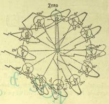
Clock Diagram, showing under swing, with perfect ankle motion obtained by use of Ramsey Swinging Pedals.
