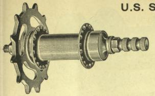
No. 996. "U.S. Standard" turned from bar, cups and cones turned, hardened and ground, dust proof bearings, finest grade nickel-plating, sprockets 7 to 12 tooth for  $\frac{3}{16}$ " chain.
