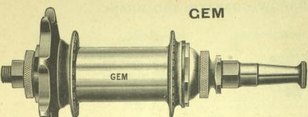
No. **999.** "Gem," turned from solid bar, cups and cones dust proof and made from special cone steel, fitted with ball retainer, has a reservoir of oil, in which the balls constantly revolve, chain line  $1\frac{1}{2}$ " or  $1\frac{5}{8}$ ", sprockets 7 to 12 tooth for  $\frac{3}{16}$ " chain.
