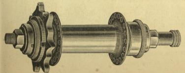
No. 1000. "Beats All," made from solid bar, cups and cones turned from best Cast Steel and accurately ground, new device for oiling hubs at both ends, chain line  $1\frac{1}{2}$  or  $1\frac{5}{8}$ , sprockets 7, 8, 9 or 10 tooth for  $\frac{3}{16}$  chain.
