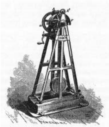
Figs. 7 and 8: Thurston's Autographic Tester and Mayer's Chromatic Photometer
