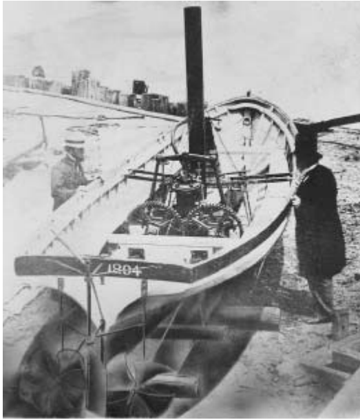
Fig. 1: The Little Juliana , with original boiler & engine in a reproduction of the boat.
