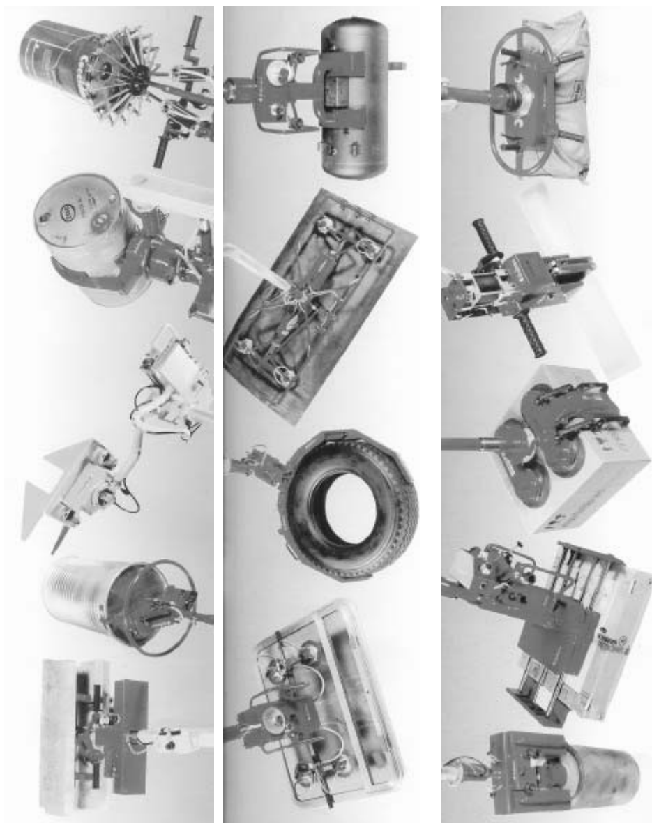
Fig.9: Grippers of manipulator «dalmec» (Italy).
