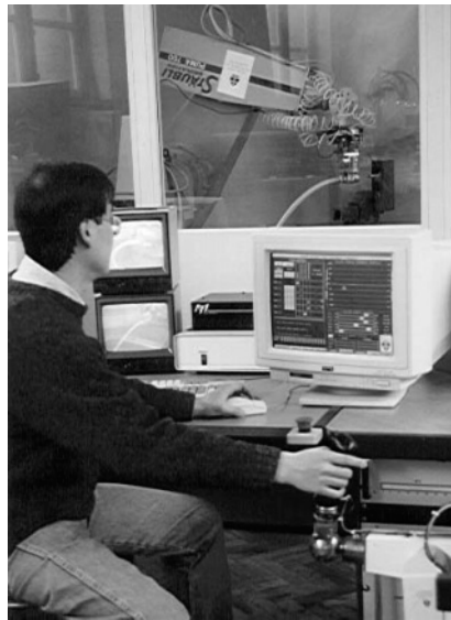
Figure 11 - Newcastle advanced 6-axis force reflecting tele-robotic system
