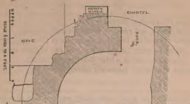
Plan of Jamb of Chancel-arch, and part of Round Tower, Finghin's Church, Clonmacnoise, (showing Norman mouldings cut on the same stone which forms part of the original construction).
