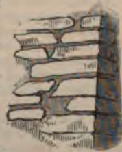
Masonry of Round Tower taken at the door.
